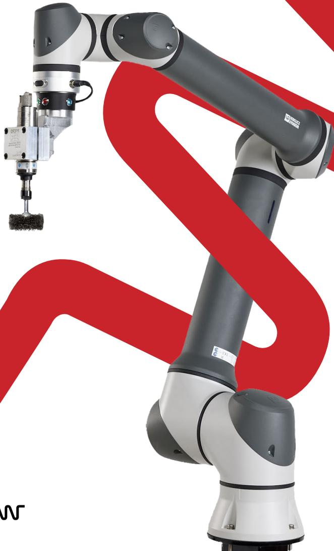
An automated brushing system for surface preparation, ensuring consistent finishes that enhance product quality.
