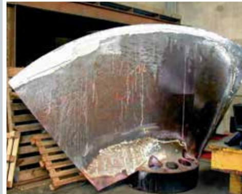
Kaplan turbine blade TETRA V 309L-G + CAVITALLOY
