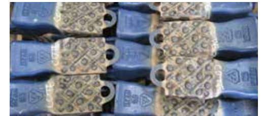
Bucket teeth made with spot welds and grid passes
