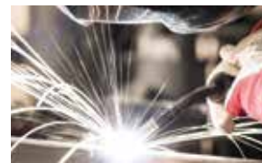
Gas shielded metal arc welding
