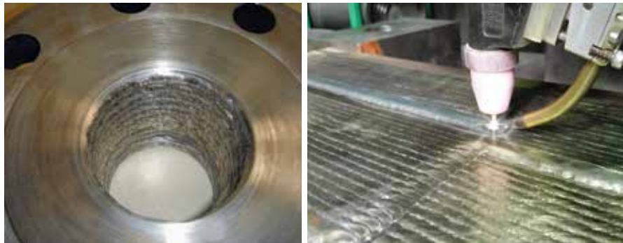
Flange borehole cladded with STELLOY 6-G. Automatic weld overlay using TIG hot wire process (STELLOY 6 TIG)
