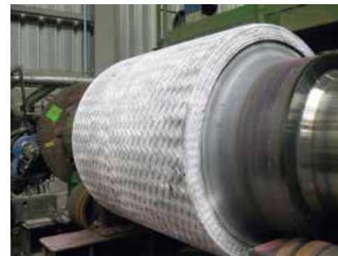
Roller press with chevrons for crushing.
