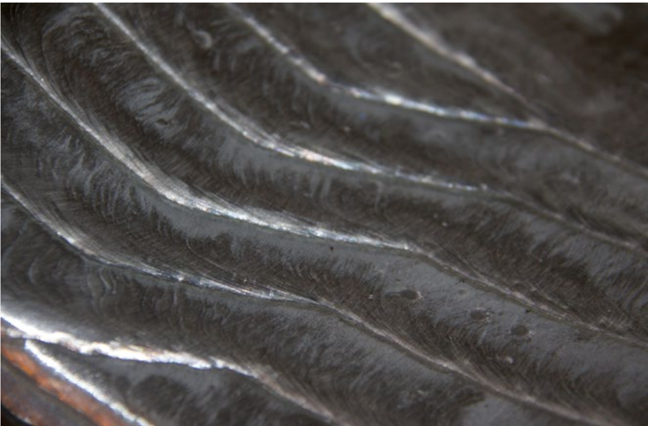
Strip cladding: BF 46 / BA-Strip 625 / Size: 60 x 0.5 mm (picture 1) and 30 x 0.5 mm (picture 2)
