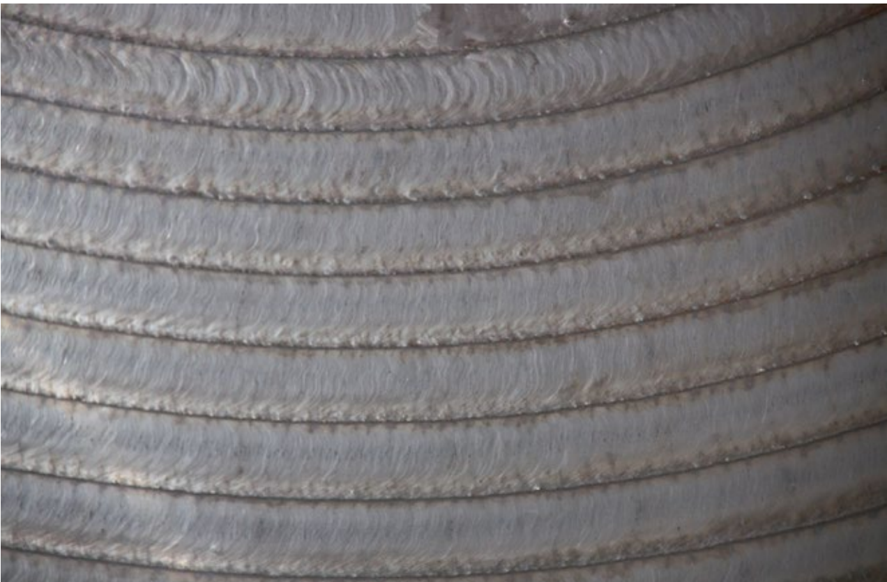
Strip cladding: BF 44 / BA-Strip 309LNb / Size: 60 x 0.5 mm
